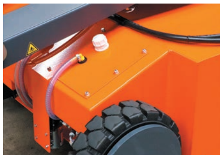
Machine casing with integrated water tank and level indicator
